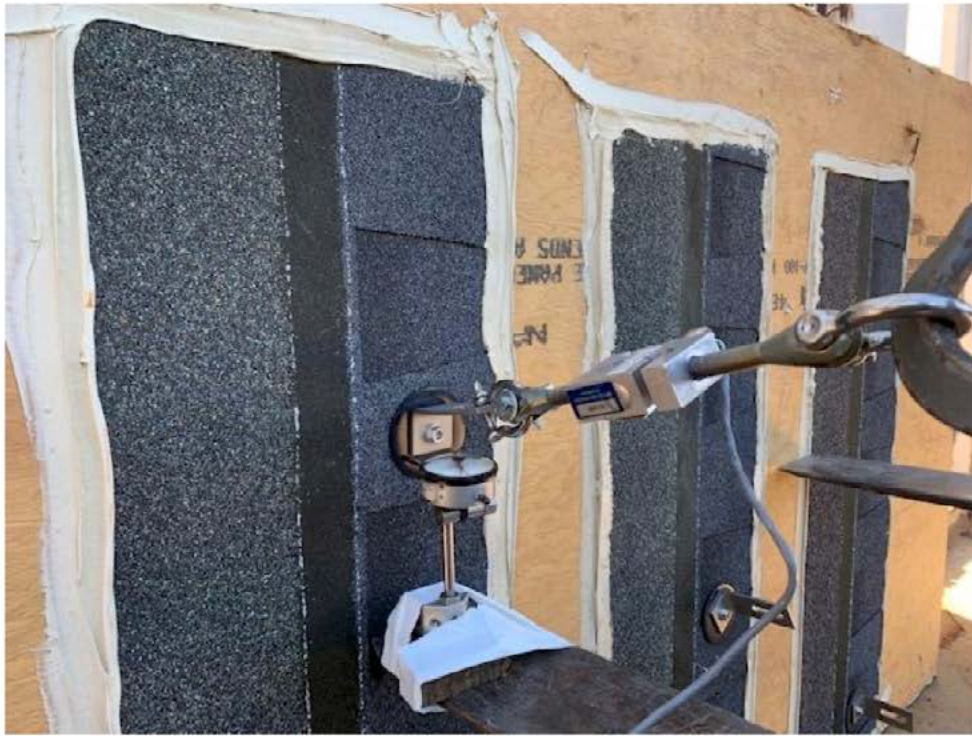
Photo No. 1 Pullout Test
