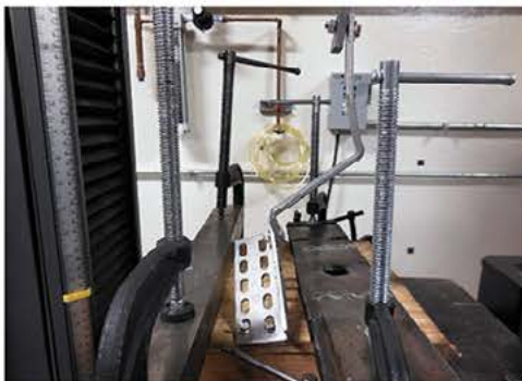
Photo 3: Typical Failure Mode - Fastener Pullout
