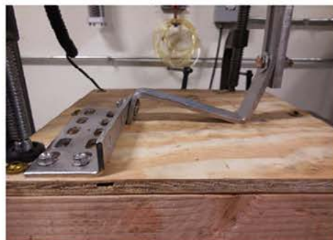
Photo 8: Typical Failure - Contact with Plywood
