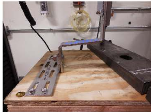
Photo 6: Compression Test Setup
