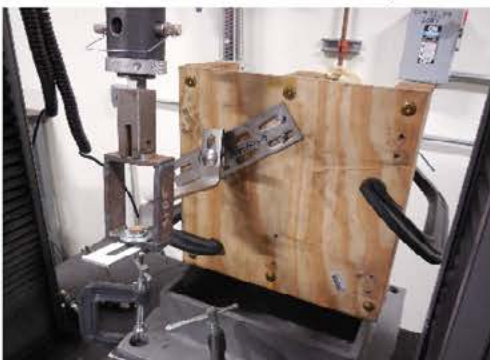
Photo 11: Deformation of Hook at Weld
