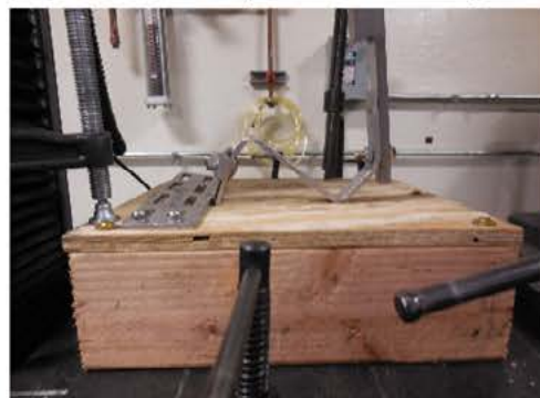
Photo 8: Typical Failure - Contact with Plywood
