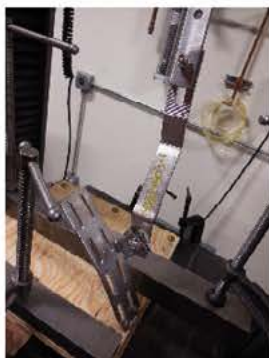
Photo 3: Typical Failure Mode - Fastener Pullout
