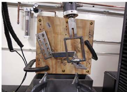
Photo 11: Deformation and Rotation of Hook
