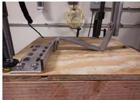
Photo 8: Typical Failure - Contact with Plywood
