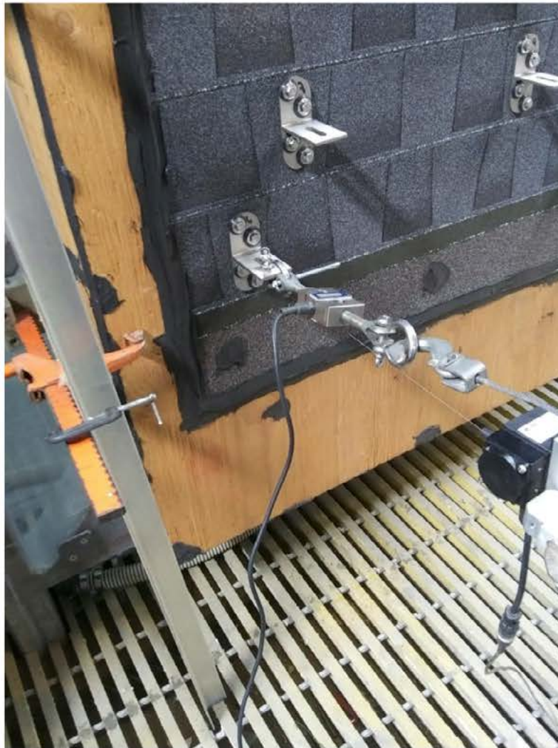
Photo No. 1 Pullout Test
